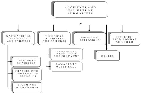
Fig.1. Division of submarines accidents and failures
