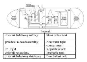
Fig. 7. Scheme of submarine model's compressed air system [4]:1 - cylinder with compressed air, 2 – linear filter, 3 – reducing valve, 4 – safety valve, 5 – ball valve, 6 – cylinder charging terminal, 7 – electromagnetic valves, 8, 9 – air distribution station, 10 – low pressure conduits, 11 – high pressure steel conduit, 12 – bulkhead passage for air conduits
