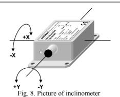
Voltage makes an output signal from the inclinometer. The voltage is registered via a measuring card installed in the computer and recalculated onto the angular scale. Signals gathered from the sensors are transmitted by conductors to the computer to be displayed on the monitor in a form of ready parameters of the watercraft's position.
