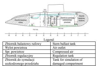
Zbiornik balastowy dziobowy Bow ballast tank Fig. 4. Scheme of ballast system and location of tanks in model?a bull
