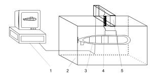
Fig. 2. Scheme of stand for tests on stability and unsinkability of submarine's model:1- operator's stand, with computer controlling and
